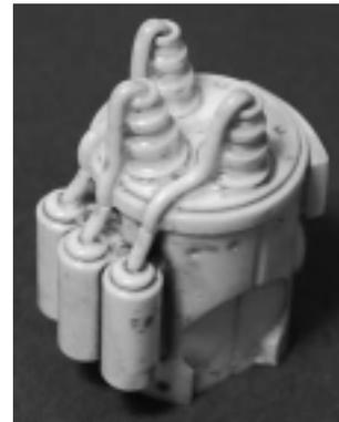
Glue the top onto the body. Make sure that the cables line up from the top to the batteries.
