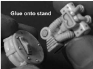
Glue this main body onto the stand. You will see where the round part of the motor fits onto the base. Slide the body up as far forward as it will go.
