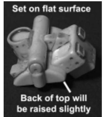
Glue the back of the bot against the flat part of the top. Do this while setting it on a flat surface. The top of the robot will be at an angle when you do this.
